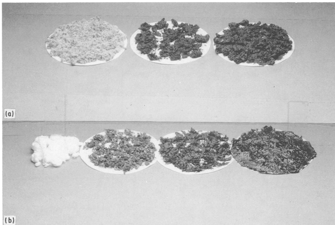
Figure 3 Evaluation of the binding of the fibres to bitumen. (a) Cellulose fibre 2, (b) glass 8.
